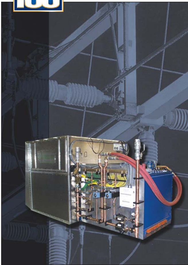
The Polyphase Converter-Modulator (foreground) is the next-generation high-voltage, high-power system — a system that generates 140-kilovolt pulses at 11-megawatt peak power and 1.1-megawatt average power. This system does most of its work at low voltage and generates high voltage only when needed — which significantly improves safety and efficiency.
